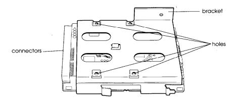
The bracket on the mounting plate should be on the opposite side of the connector end of the drive.
